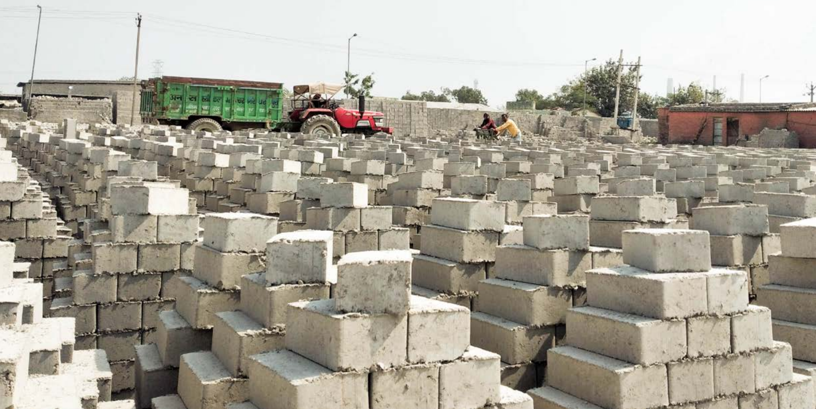
Image Description: Fly ash bricks at a factory located in the RIICO Paryavaran Industrial Area, Kota
